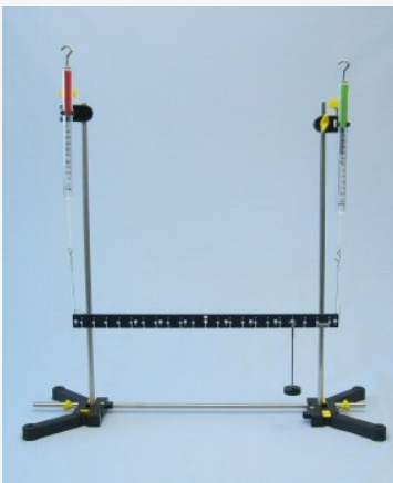
Test setup for determining support reactions
